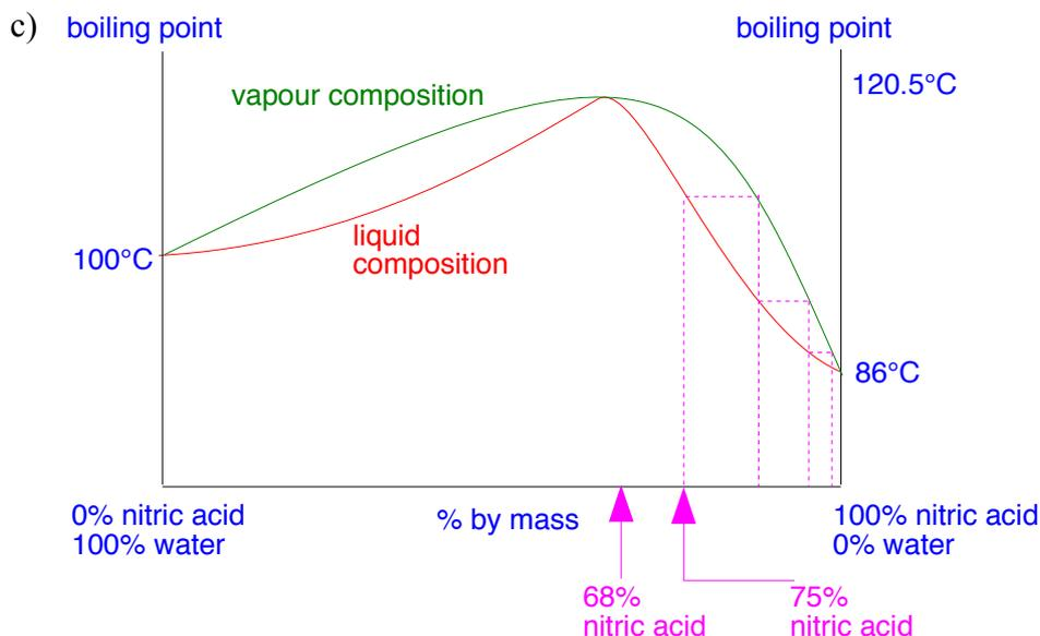
This time, on boiling, the vapour is richer in nitric acid. If you condense this, and boil it again, the vapour will be even richer in nitric acid. That means that by carefully controlling the temperature, you will be able to get pure nitric acid out of the top of the fractionating column.
