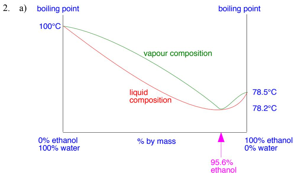
b) An azeotropic mixture is one which has a constant boiling point, and where the vapour over the top of the liquid has exactly the same composition as the liquid itself. If you boil such a mixture, it will simply boil away with no change in boiling point, just as if it was a single pure substance.
