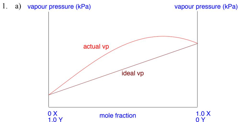
You don't actually need to include the ideal vapour pressure line. It doesn't matter where you draw the maximum point of the actual vapour pressure curve - but it should have a maximum higher than the vapour pressure of X. If you drew this curve with a minimum rather than a maximum, remember that a **positive** deviation from Raoult's law means that the **vapour pressure** of a mixture is always **higher** than ideal.
