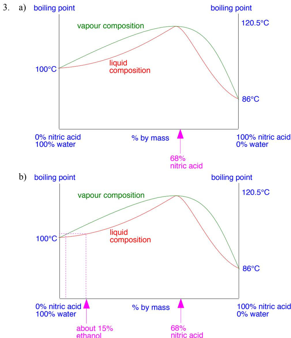
If you boil a mixture containing 15% nitric acid, it will produce a vapour richer in water. Condensing and reboiling this will soon lead to pure water at the top of the fractionating column. As the liquid loses water, it will gradually become more concentrated until it reaches the azeotropic mixture, at which point there will be no further changes in its composition. The flask will eventually contain the azeotropic mixture.
