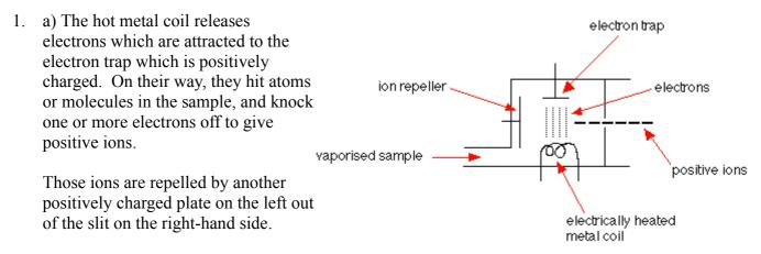
b) The ionisation chamber is held at +10,000 volts. After leaving the chamber, the beam passes through two more slits, the last of which is at 0 volts. The positive ions are accelerated by repulsion from the very positively charged ionisation chamber.
