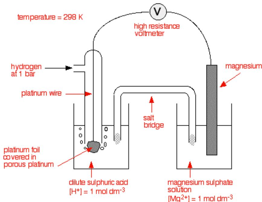
Be sure that your diagram contains all of the above labelling, including the conditions, and the fact that the voltmeter has to have a high resistance.
