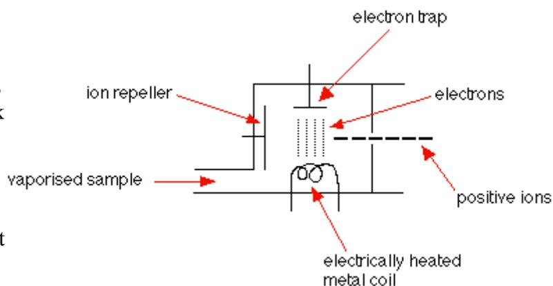
Those ions are repelled by another positively charged plate on the left out of the slit on the right-hand side.
